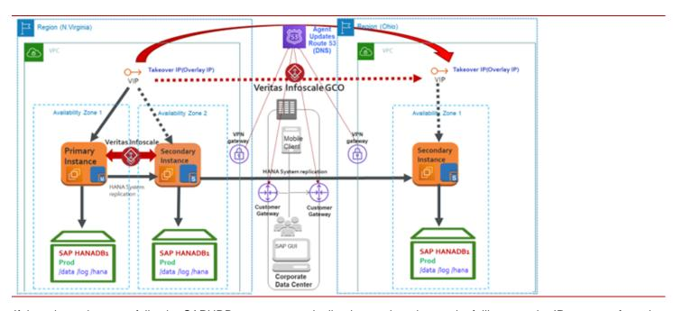
If the primary instance fails, the SAPHDB agent automatically triggers the takeover by failing over the IP resource from the primary to the secondary instance in the same region. Virtual IP failover operations are managed by the AWSIP and the IP agents. The following graphic shows how the secondary becomes the primary and is active in AvailabilityZone2:
