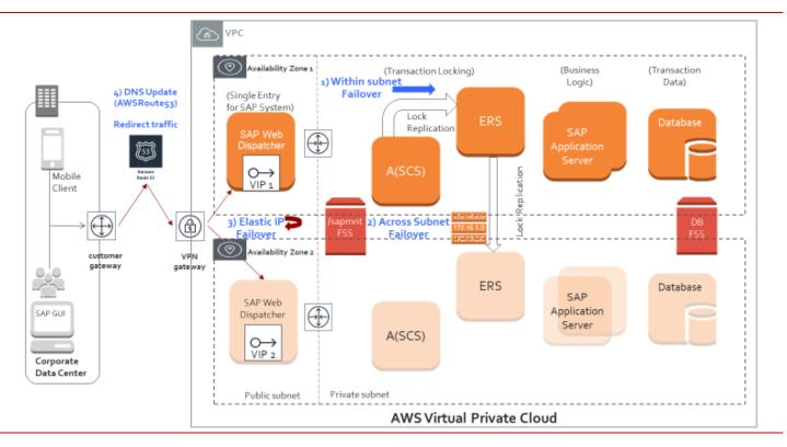
In addition to configuring SAP HANA for HA, DR, or both HA and DR, you need to ensure that the client applications (i.e. the S/4HANA/NetWeaver application server, JDBC, ODBC connection, and so on) can re-establish their connection with the SAP HANA database after the failover. To do so, you can configure either network-based IP redirection or network-based DNS redirection of your SAP HANA system. The InfoScale agents for SAP support end-to-end HA and DR for SAP NetWeaver and SAP S/4HANA.
